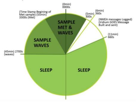
The primary mechanism to deliver observations for buoys having the WM100 payload is via satellite telemetry (GOES). Historically the MSC moored buoy programme was managed and processed by a system called WBS (Weather Buoy System), which has now been replaced by the DMS. The buoys report hourly meteorological, housekeeping and wave statistics data, which are quality assessed in real-time by the DMS. WMO and SWOB products are produced and
