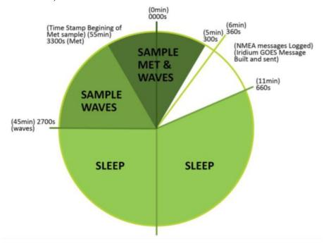
The primary mechanism to deliver observations for buoys having the WM100 payload is via satellite telemetry (GOES). Historically the MSC moored buoy programme was managed and processed by a system called WBS (Weather Buoy System), which has now been replaced by the DMS. The buoys report hourly meteorological, housekeeping and wave statistics data, which are quality assessed in real-time by the DMS. WMO and SWOB products are produced and
