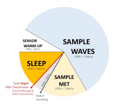
WM500 data sampling. Data samplings begins 45 minutes after each hour for a duration of 20 minutes (ending 5 minutes after each hour) and message transmission 1 minute later (6 minutes after each hour):
