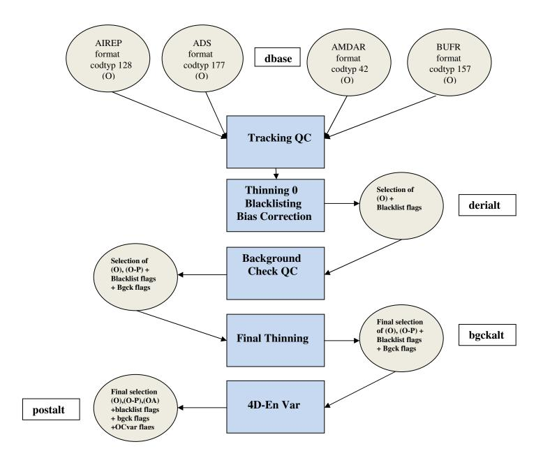
Figure 1: Aircraft observations processing; Operational branch, last file is in postalt directory.
