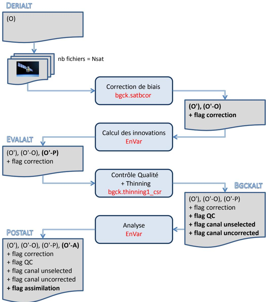
**Processing of GeoRad radiances.** Gray wavy bottom edge rectangles represent BURP files while blue rounded corners rectangles represent processes (with the program names in red).
